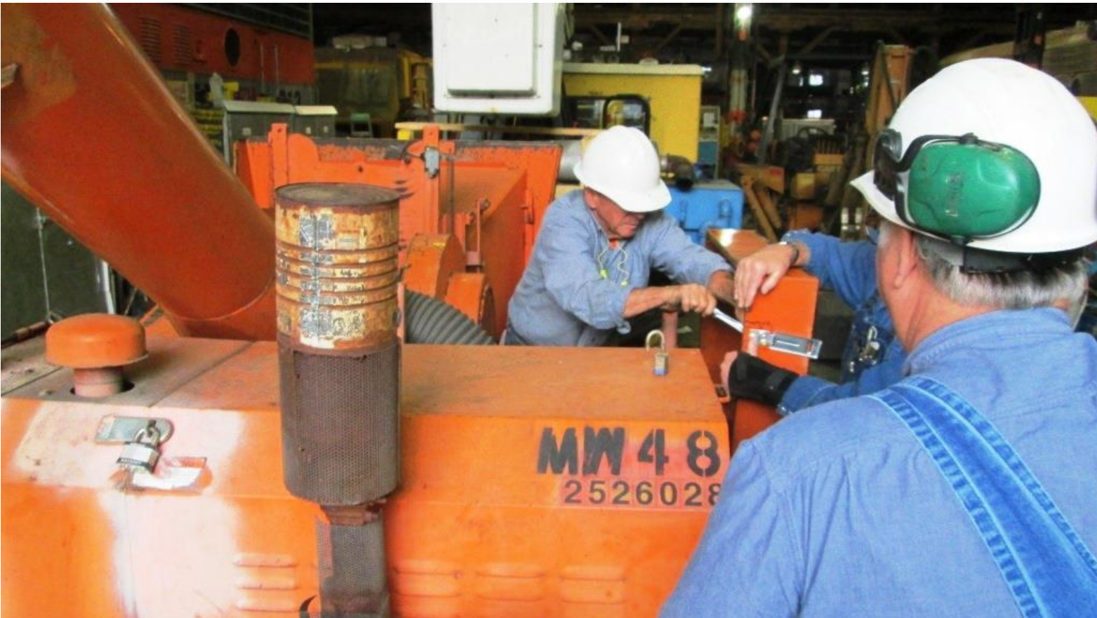
Mike T. makes final adjustments to the chipper's batter box
